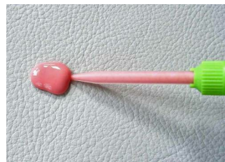
Mixing the components in the mixing tip
